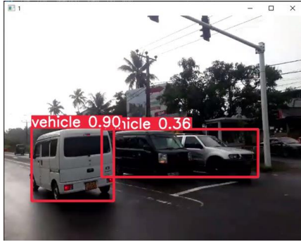
Figure 3: Vehicle Detection at Day Time from Camera One.
